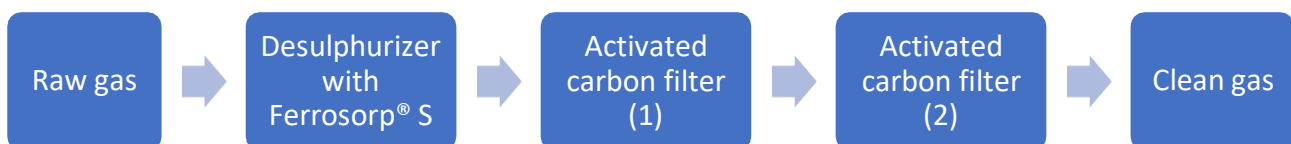
Figure 3: The process flow diagram of the desulphurization process in the watertreatment plant
